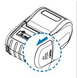
Push the Open into the direction indicated with the arrow in the image.
