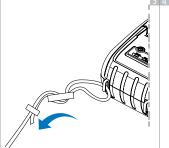
After pulling out the end of strap tightly, put it into the clip to be fastened.
