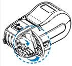
Open the battery cover and push up the hook to the direction as above.
