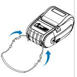
Insert the strap into the hook on the printer.
