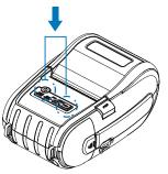
While you are pressing the FEED button, press the power button
