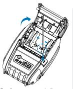
Open the paper cover pressing the open button. Insert a sharp tool into the paper guide hole and push it in the direction of arrow as shown above.
