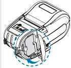
Close the battery cover once you inserted the battery completely.
